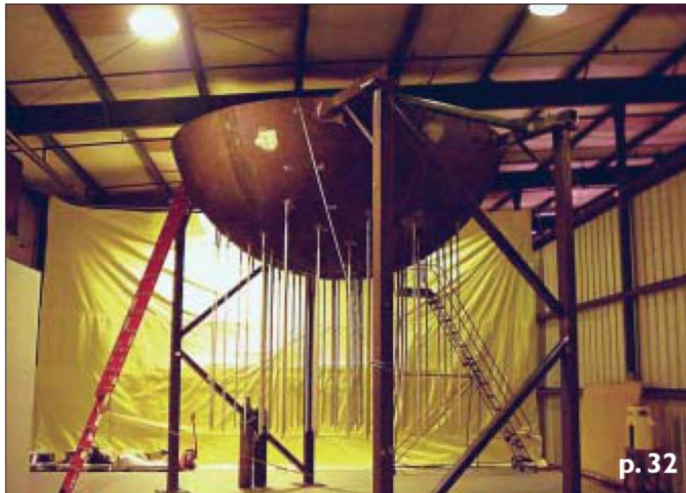
Figure 5 – Full Scale Mockup Used at STP-1 (Nuclear News, October 2004)
